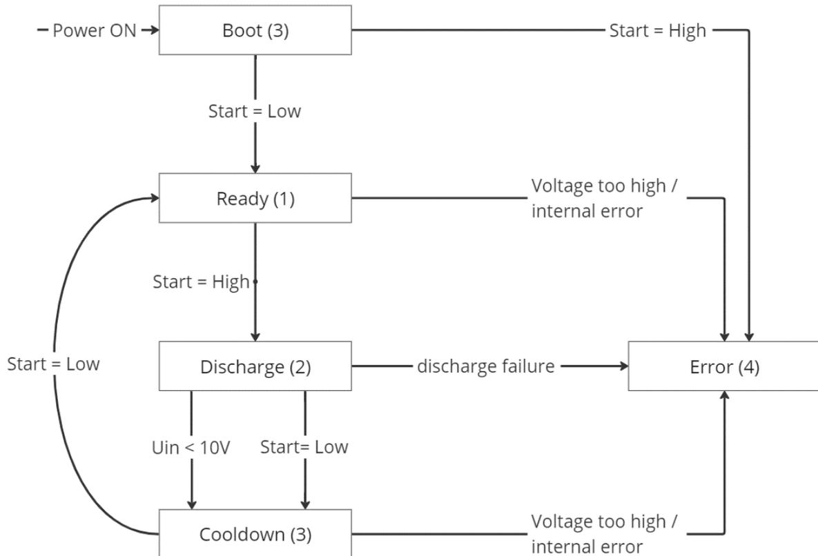
After the boot procedure, the device switches to the ready state (applying the Start signal before powering up the device leads to an error).
