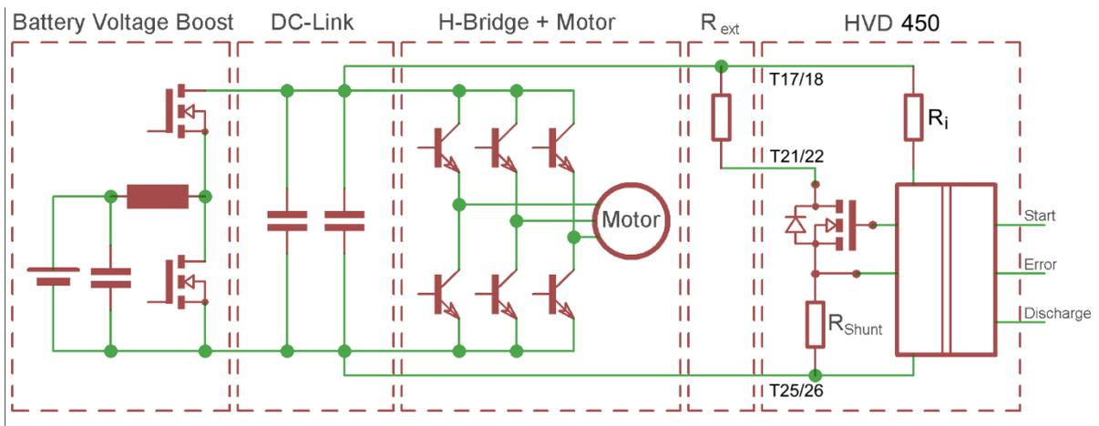
Figure 5: connection of HVD 450 to DC Links
