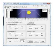
Commander has an artificial daylight program. This can control fluorescent or LED lamps with analogue or DALI signals.
