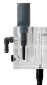
*FluoriSense in a single open flow cell*
