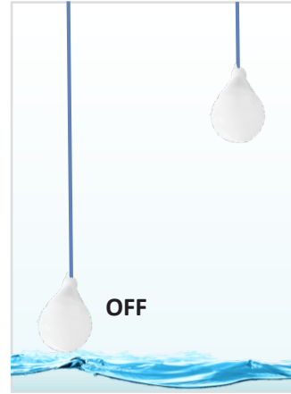
The pumping stops as soon as the low regulator returns to the vertical position
