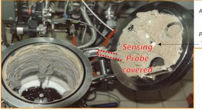
A small batch reactor still operating efficiently with the probe totally covered in product build-up
