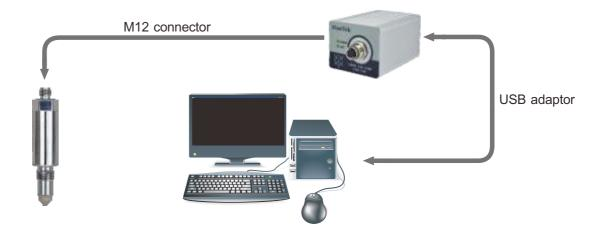
Using M12 connector to link SIS Impedance Spectroscopy Sensor" with programmer box. Transmitting the sensor data by USB cable from programmer box to PC. Note: The accuracy and efficiency can not be guaranteed if using NON-FineTek connector.
