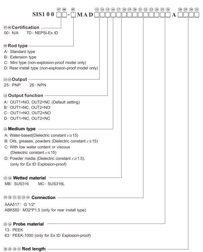
CodeLength004747mm(Standard or Mini type)007272mm(Extension type)002929mm(Rear install type)
