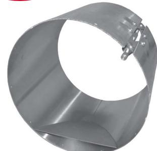
Use optional VD stainless steel Pipe Dam Bands downstream from an area-velocity sensor installation to maintain low flow water level at 1" (25.4 mm) or higher as required for ultrasonic level measurement.
