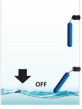
The liquid reaches the float The pumping stops as soon as vertical position
