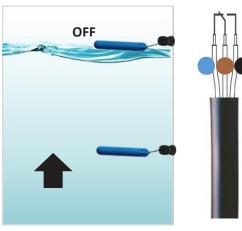
The filling stops as soon as the high level regulator switches
