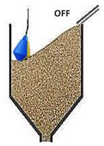
When the high level is reached, the level sensor tilts and stops filling the silo
