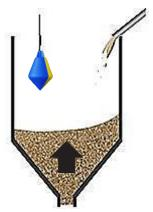
When the silo fills up, the level sensor is suspended vertically.
