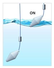
The liquid reaches the float which by tilting gives the signal to the pump to start for emptying
