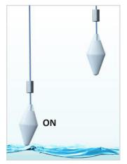
The filling starts as soon as the low regulator returns to the vertical position
