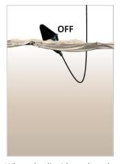
When the liquid reaches the float, it tilt shut off the power to the pump
