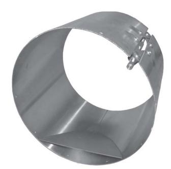
Use optional VD stainless steel Pipe Dam Bands downstream from an area-velocity sensor installation to maintain low flow water level at 1" (25.4 mm) or higher as required for ultrasonic level measurement.
